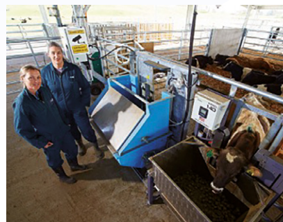
A photo of the feed intake and GreenFeed methane machine in the Young bull methane trial.
